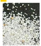
Lane Mountain Silica Sand is a high quality, high purity, close graded white silica sand. Lane Mountain Silica sand is suitable for sandblasting steel, concrete and wood and as an additive for white plaster, mortar or concrete. Available in six grades: LM #16, LM #20-30, LM #30, LM #50, LM #70, LM #125
