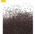
STARBLAST® blasting abrasives are a loose blend of coarse and fine staurolite sands that are uniformly sized and have clean, rounded surfaces. Mined from mineral deposits in Northeast, Florida, the naturally occurring sands are scrubbed and chemically washed to ensure freedom from dirt, dust, and ultrafines.
