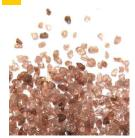
Garnet is a naturally occurring almandite garnet, the hardest of all known garnet types. All grades have a Moh's hardness of 8, with a specific gravity of 4.1. Garnet is available in size grades to meet requirements for any project. Grade sizes are: # 12-25, # 20-40, #30-60, # 50-80, # 80, #120
