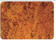
KEY: Steel where all mill scale has flaked KEY: Steel where pitting and complete off and complete rusting has taken place rusting has occurred
