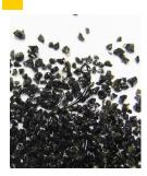
TARGET® Black Magic is an abrasive grit prepared by selective screening of coal slag to give a series of clean, sharp abrasives meeting the requirements of the abrasive blast cleaning industry. The product meets the requirements for classification as a Type I Inorganic Material under U.S. Military Specification MIL-A-22262A (SH). Available sizes are: 16-40, 20-40, 40-60
