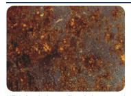
KEY: Steel where mill scale has started to flake and light rusting occurs
