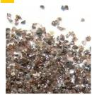
Aluminum Oxide grits are the most efficient blasting media. It is the fastest cutting product used for industrial blasting and surface preparation, due to its extreme hardness of 9 on Moh's scale. Aluminum Oxide is a manufactured material, electrofused from bauxite and is exclusively produced for Target Products Ltd.. Grit sizes available: 16, 24, 36, 54, 70, 100, 220
