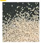
K2-Strip is an odourless, non-sparking, non-volatile, non-flammable and non-controlled substance. It is water soluble. No special disposal considerations are required.
