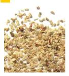
Corn Cob is the choice when the job calls for softer, less dusty and an environmentally safe abrasive. This blast cleaning media is suitable for metal, wood, fibreglass, plastic, masonry, electrical insulators and other sensitve materials. It is non-sparking and safe to use around gears and hydraulic rams. Available size is 20-40.
